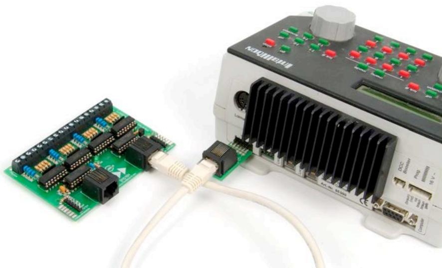
It is recommended to use the s88-N adapter (sold separately). This small adapter changes the standard S88 connection on your central unit into a s88-N connection. Instead of a normal S88 cable, you can now use a reliable and inexpensive network cable to connect your first decoder.
